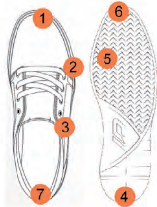
Figure 2. The most common areas of damage to skateboard footwear
