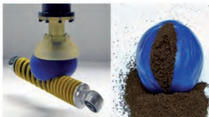
Figure 4. Tool gripper with coffee grounds
