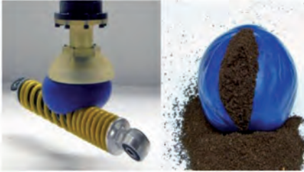
Figure 4. Tool gripper with coffee grounds
